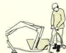
FULL RANGE OF OPTIONAL EQUIPMENT ALL POWERED FROM HYDRAULIC POWER TAKE - OFF
