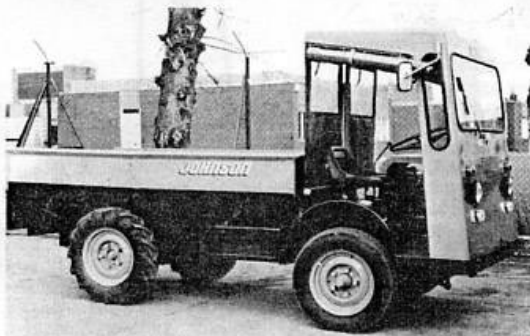
With a 7.5 hp single-cylinder air-cooled diesel engine, this Johnson "Motil" lightweight utility truck has a top speed of 14.3 kph and can carry a 1,334kg, 1.9m 3 load and represents Johnson's most recent innovation.
