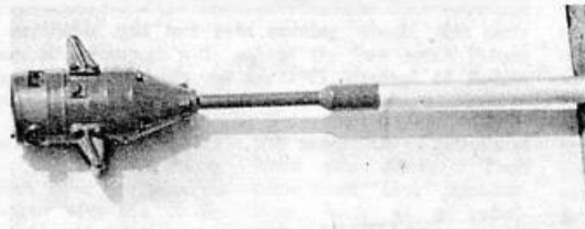
In the late 'thirties, this pioneer, rigid-shaft electric vibrating poker was a Johnson innovation, soon followed by another, the flexible-shaft version, claimed to be the first in the UK.
