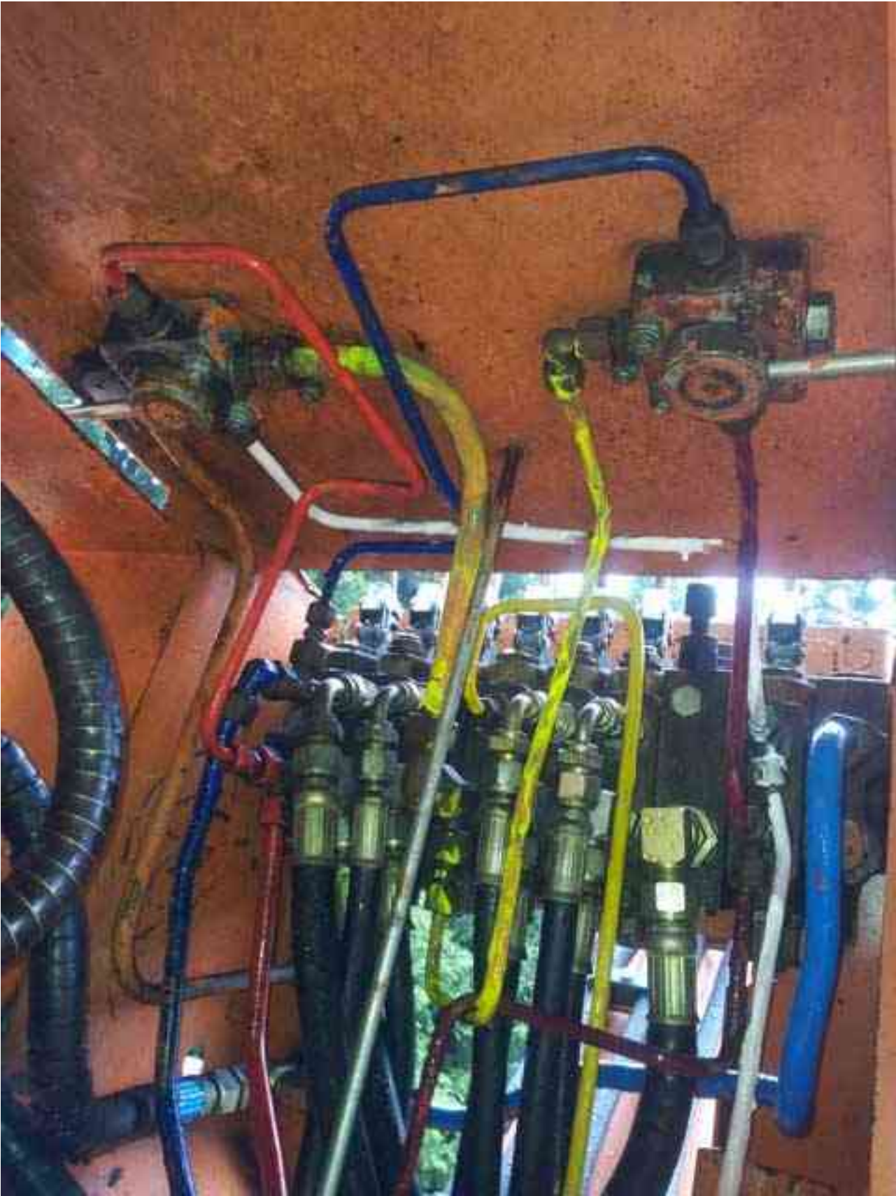
Powerfab 360WD (three wheel version) colour coded hydraulic layout by Uli.
