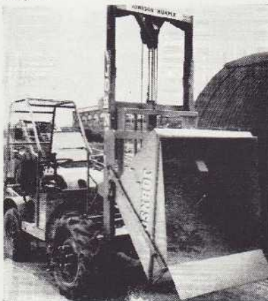
As a high-discharge, hydraulic tipping dumper. Ground clearance when fully tipped 7 ft. 6 in.
