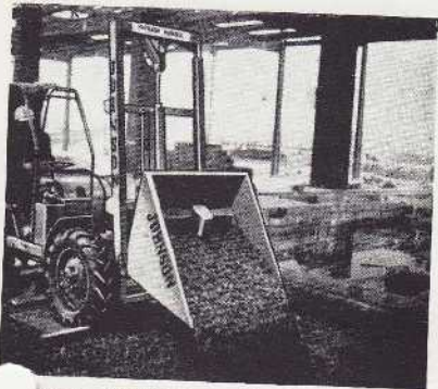
Humper — Maximum discharge height — skip tipped — 7 ft 6 in
